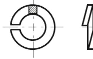
*Spring lock washers for screws with cylindrical heads*
